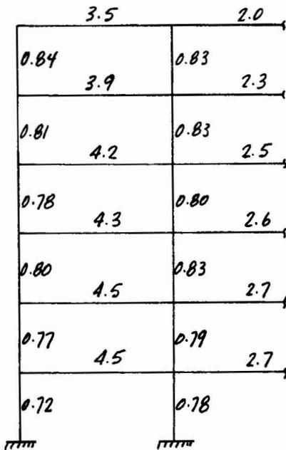
Fig. 4b. Modified substitute structure analysis: damage ratios.
