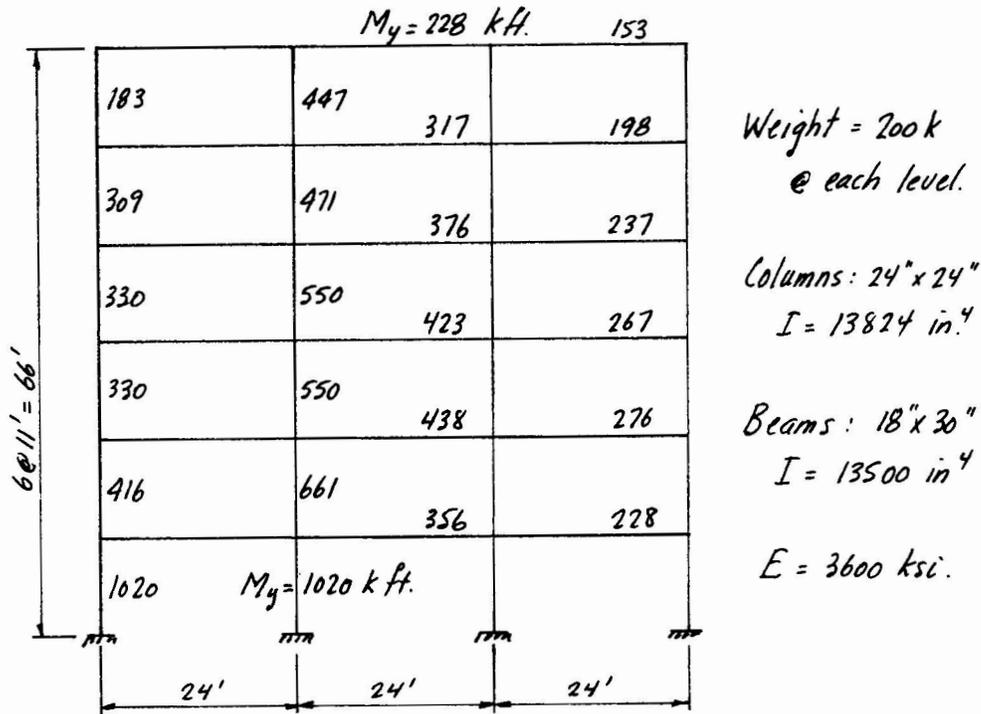
Fig. 4a. Symmetric 3-bay, 6-storey frame: layout, member properties, weight.
