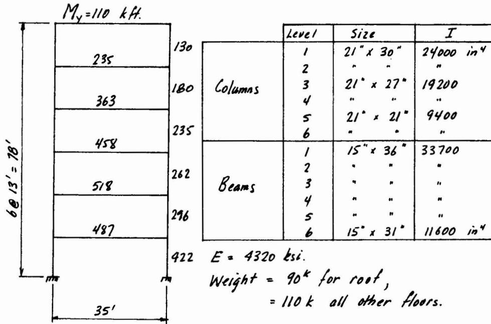
Fig. 6a. 1-bay, 6-storey frame: layout, member properties, weight.
