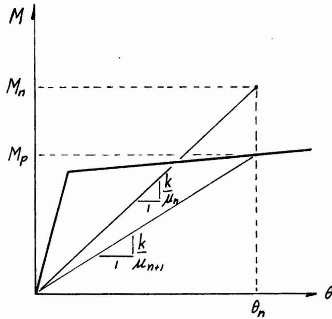
Fig. 2. Moment curvature relationship: damage ratio iterations
