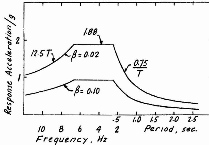
Fig. 3. Acceleration response spectrum: smoothed average of six earthquakes normalised to  $A_{\max} = 0.5g$ .
