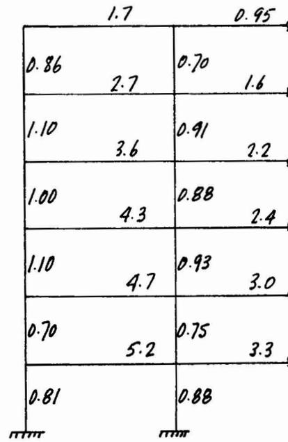
Fig. 4c. Nonlinear dynamic analysis: average damage ratios
